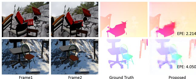
Fig. 5. Examples of optical flow prediction on MPI Sintel final dataset. We show both results with/without fusion unit. Fusion unit successfully improves the prediction. Some noise are removed and prediction errors are corrected.
