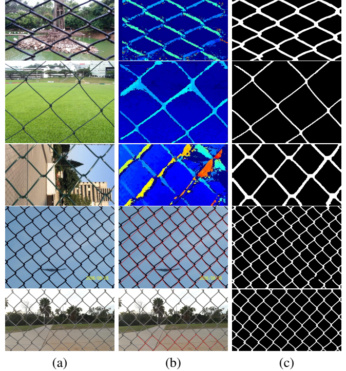
Fig. 6. Comparison of fence segmentation. (a) input images; (b) estimated disparity by [9] for the row 1–3 and detection results by [1] for the row 4–5; (c) results by the proposed method. Input images are from [1, 8, 9, 12] and our test set.
